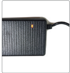
④ Red light shows the battery is charging, green light is full
