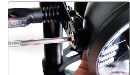
Attach the light to the screw and tighten it
