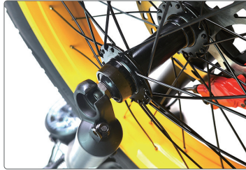
Turn the car upside down. Install the side with the ebike disc into the direction with the disc brake
