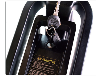
Turn the key clockwise to unlock the battery lock, then push it forward
