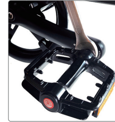
Tighten the left pedal "R" counter clockwise
