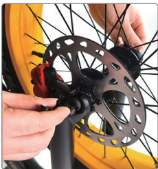
Tighten the spring and nut to the screw
