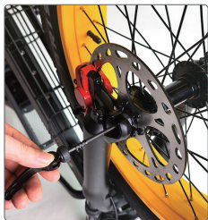
Put the quick release handle into the tire
