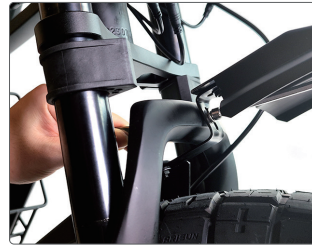
Secure the nut with a wrench and tighten the other end with a hex.
