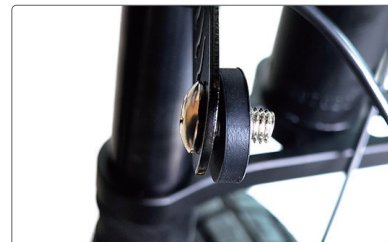
Fasten the screw fittings to the forks
