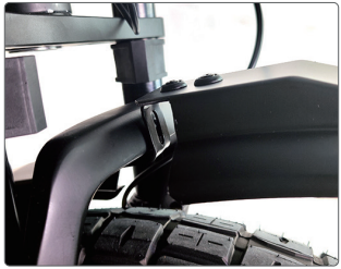
Align the fender screw holes with the screw holes on top of the fork
