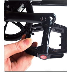
The pedal "L" is installed on one side of the chainring, and "R" is opposite to the chain ring
