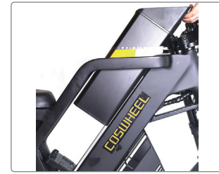
Pull out the battery by hand
