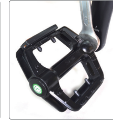
Tighten the right pedal "L" clockwise
