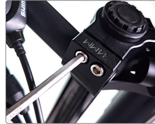
Loosen the screws on each side
