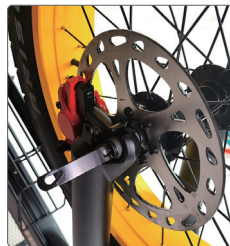
Press the quick release lever handle down
