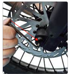
Tighten the nuts to complete the installation.
