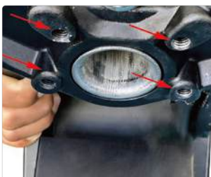
Tighten each screw into its corresponding hole.
