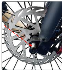
Insertion of quick release lever
