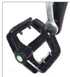
Tighten the right pedal "R" counter clockwise
