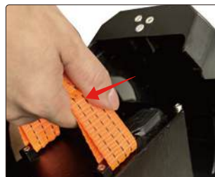
Lift the battery upward.
