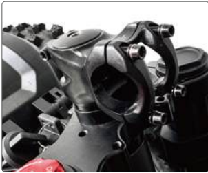
Remove these 4 screws first
