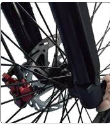
Putting the tyre into the fork slot
