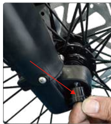
Tighten the screw cap on the other end of the quick release lever
