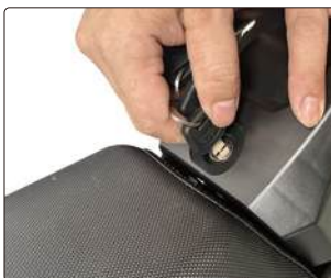
Open the battery lock
