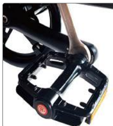
Tighten the left pedal "L" counter clockwise
