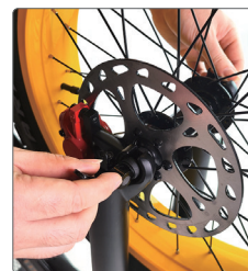
Tighten the spring and nut to the screw
