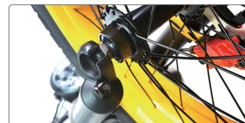
Turn the car upside down. Install the side with the ebike disc into the direction with the disc brake
