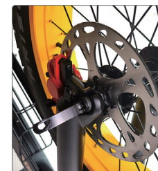
Press the quick release lever handle down
