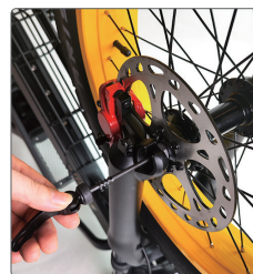
Put the quick release handle into the tire
