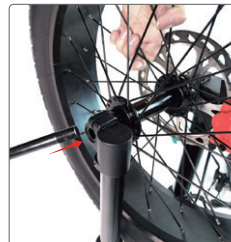
⑤ Insertion of quick release lever
