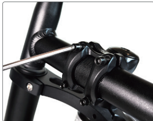
③ Fixing Direction Tighten screws
