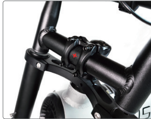
② Insert the handlebar into the adjustment position and cover the catch
