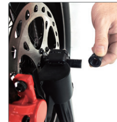
⑥ Tighten the screw cap on the other end of the quick release lever
