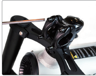
① Remove these 4 screws first
