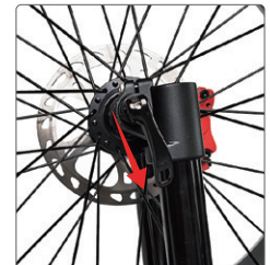
⑦ Lock the quick release handle to complete the front wheel installation
