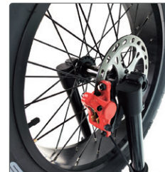
④ Putting the tyre into the fork slot
