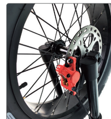
Putting the tyre into the fork slot
