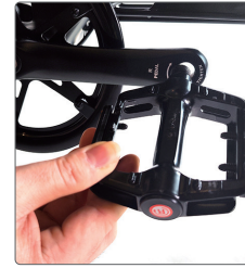
The pedal "L" is installed on one side of the chainring, and "R" is opposite to the chain ring
