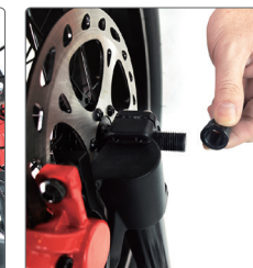
Tighten the screw cap on the other end of the quick release lever
